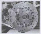
With the rear wheel off, the rear brakes' alloy hubs and floating disc mountings are visible scrumptious stuff for well-heeled gearheads.
